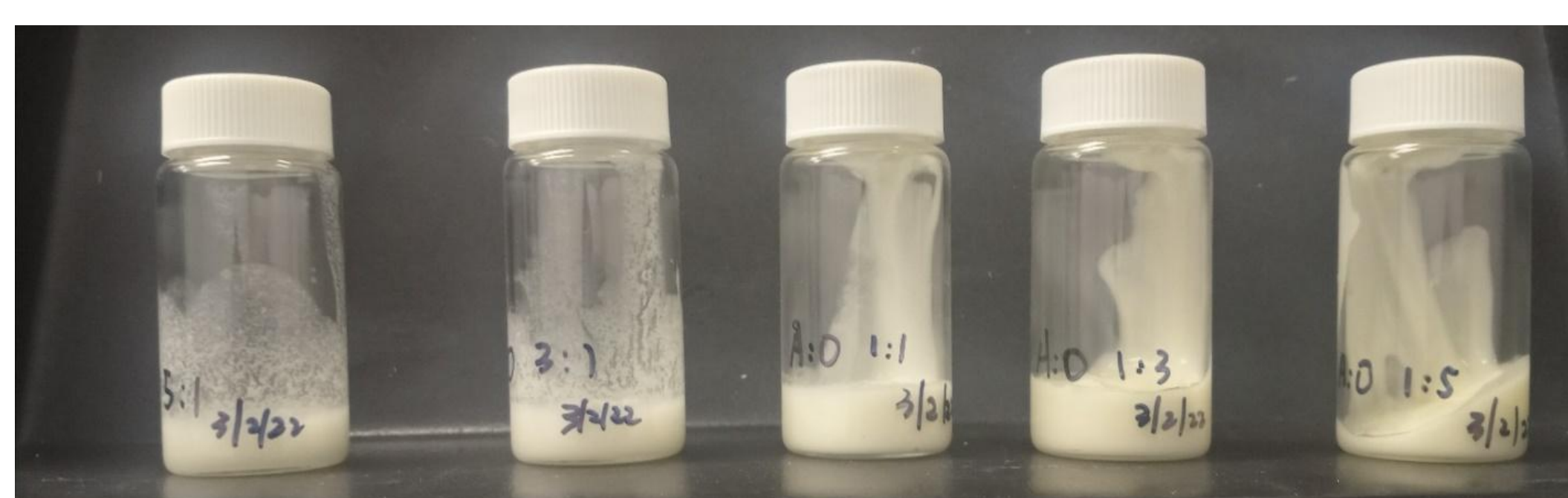
Figure 1. Bigels at five different phase ratios (left to right), A: O = 1:1, 1:3, 1:5, 3:1 and 5:1.
